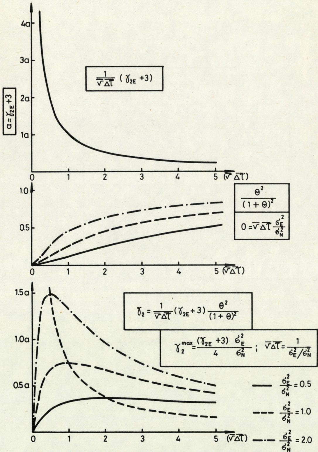
Fig.4. Dependence of  $\gamma_2$  on signal to noise relation  $\theta$  and bubble generation intensity ( $\sqrt{\Delta T}$ )
