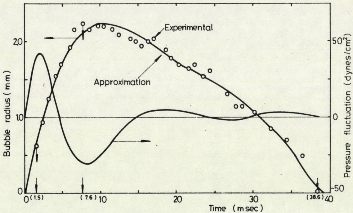
Fig. 2. Bubble history and associated pressure fluctuation (Ref [2])
