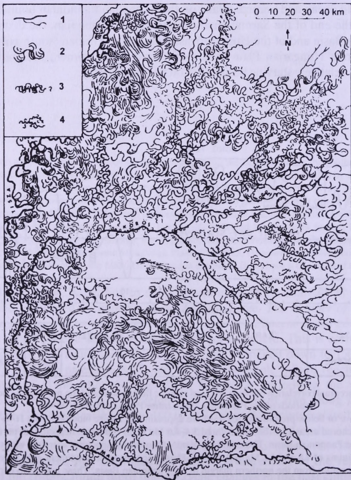
Fig. 23. Recent bed traces between Körös and Maros alluvial fans (after MIKE 1975). - 1 = present-day hydrography 2 = Tisza-size bends (amplitude = 600 m, length of arch 7 2000 m; length of chord = 1000 m); 3 = Maros-size bends, 4 = Körös-size bends
