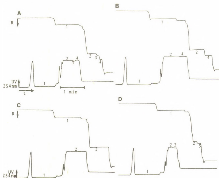
Fig. 2. Isotachophoretic analyses (electrolyte system I) of the crude material (A) and the different peptide fractions (B-D) obtained after gel chromatographic purification. Key as in Fig. 1. For each separation, 5 \mu l were injected, corresponding to 2.63 \mu g of material
