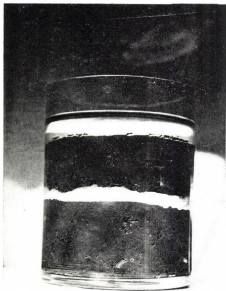
Fig. 3. Method for determination of sulphide formed by sulphate reducing bacteria in model experiment
