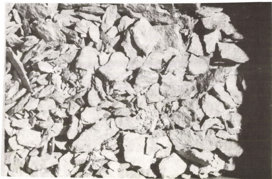
Fig. 2 Disintegrated potash-tuff of Bekecs after 180 days' freezing
