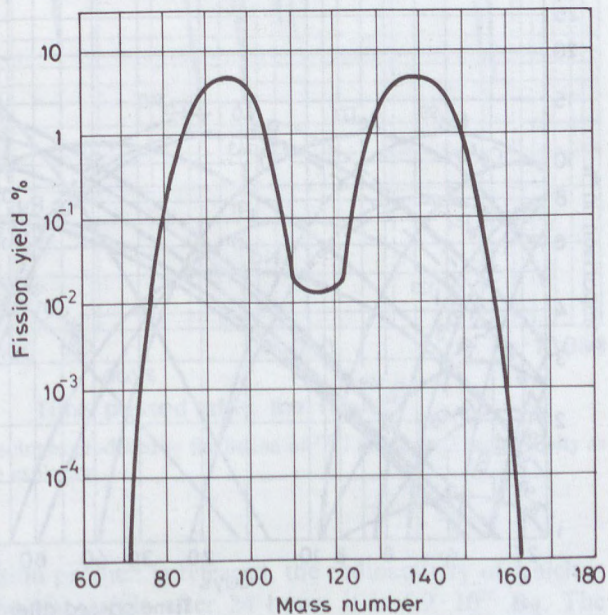
Fig. 6. Distribution of the fission products of ^{235}\text{U} as a function of the mass number
