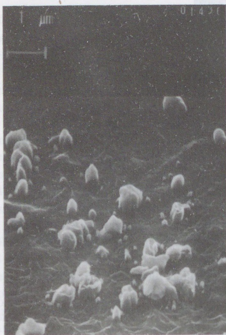
Fig. 5.10. SEM micrograph of the ion-etched surface of an impact modified PVC-sheet. (After Kalló 1979.)
