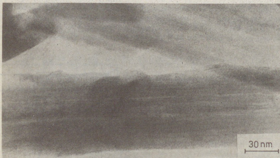
Fig. 5.22. Electron micrograph of an asbestos sample ground in a vibration mill for 4 h followed by heat treatment at 873 K for 15 min [202]
