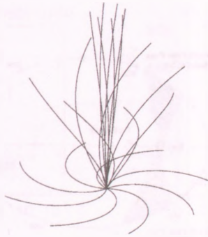
Figure 1: Schematic of Parker spiral in 3-D. The field lines are drawn for heliolatitudes 0^\circ , 40^\circ and 80^\circ , up to a distance from the Sun of 1.3 AU.
