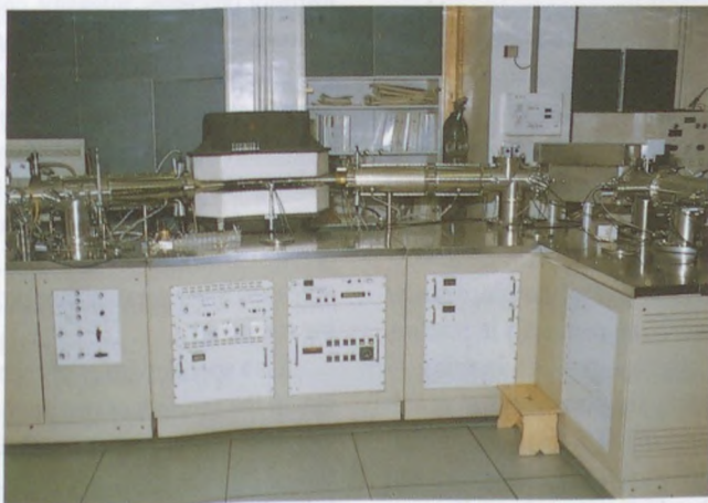
2. High resolution hybrid-tandem mass spectrometer Typ: VG ZAB-2SE0 (VG Analytical, Anglia)
