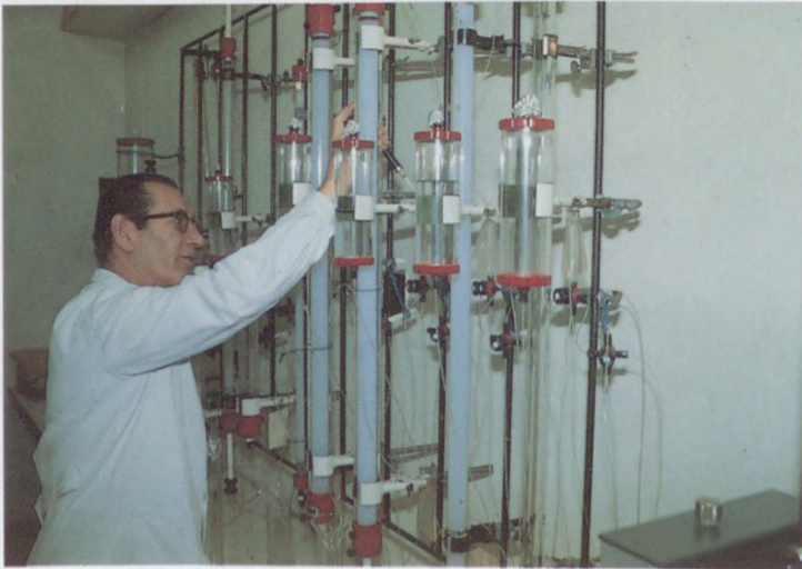
Separation of avian immunoglobulins using LKB Chromatographic System
