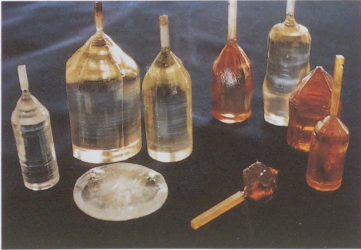
Set of optical crystals grown in the Research Laboratory for Crystal Physics from left to right: \text{TeO}_2 , \text{LiNbO}_3 , \text{LiNbO}_3\text{:Mg} , \text{ZnWO}_4 , \text{Bi}_4\text{Ge}_3\text{O}_{12} , \text{Bi}_{12}\text{SiO}_{20} and \text{Bi}_{12}\text{GeO}_{20} for side: \beta\text{-BaB}_2\text{O}_4 and \text{Bi}_{12}\text{TiO}_{20}
