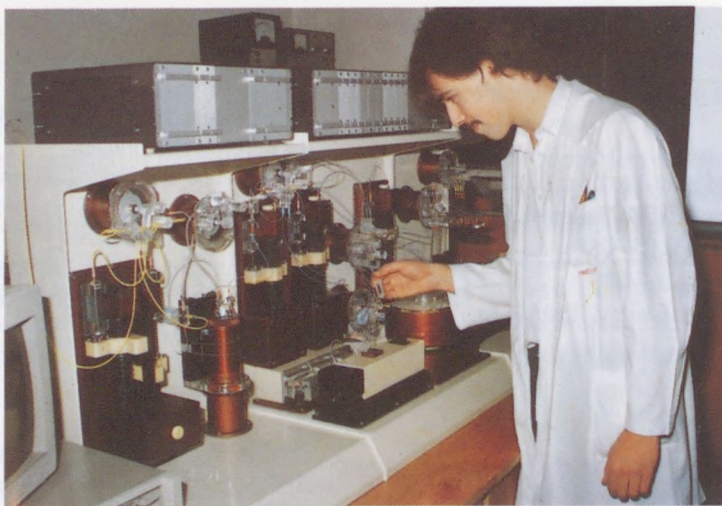
Apparatus for automatic determination of the phage-bacterium interaction parameters constructed and manufactured in Research Laboratory for Biophysics
