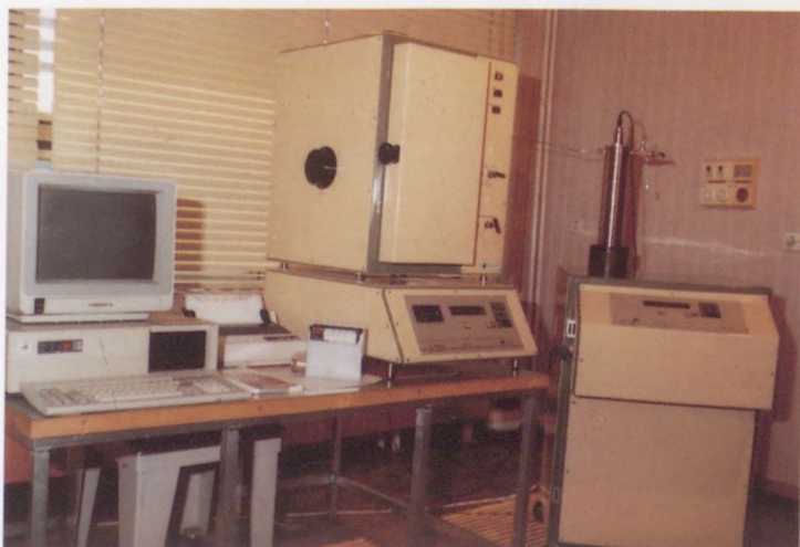
Automatic programmable PVT system for volumetric and phase study of crude oil reservoir samples under reservoir conditions.
