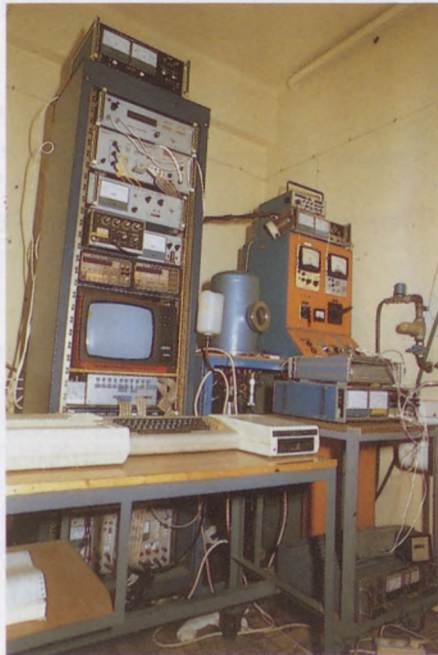
Self constructed dilatometer for creep examinations
