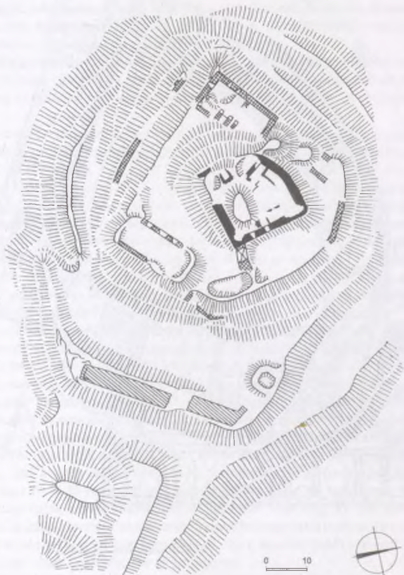
8. Templštejn, ground plan of the castle. Black shaded areas: masonry of the end of 13th century. Drawn by the author.
