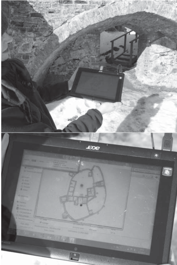
Fig. 5: The calibrated map can now be navigated in real time with a GPS-enabled tablet or laptop. Here we see the correct location in front of a castle gate. With the calibration complete, sight points can be added that will play a presentation for a user if they enter a certain radius, such as this five-meter circle that defines a single room within the building (photos by K. Uotila and E. Ernst).
