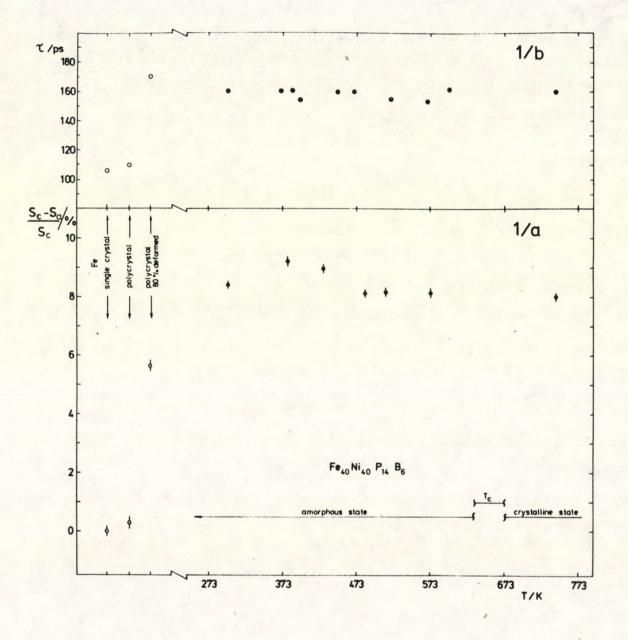
Fig.1/a. S-parameter values referring to Fe and FeuoNiuoPiuBe in dependence on heat-treating temperature;
