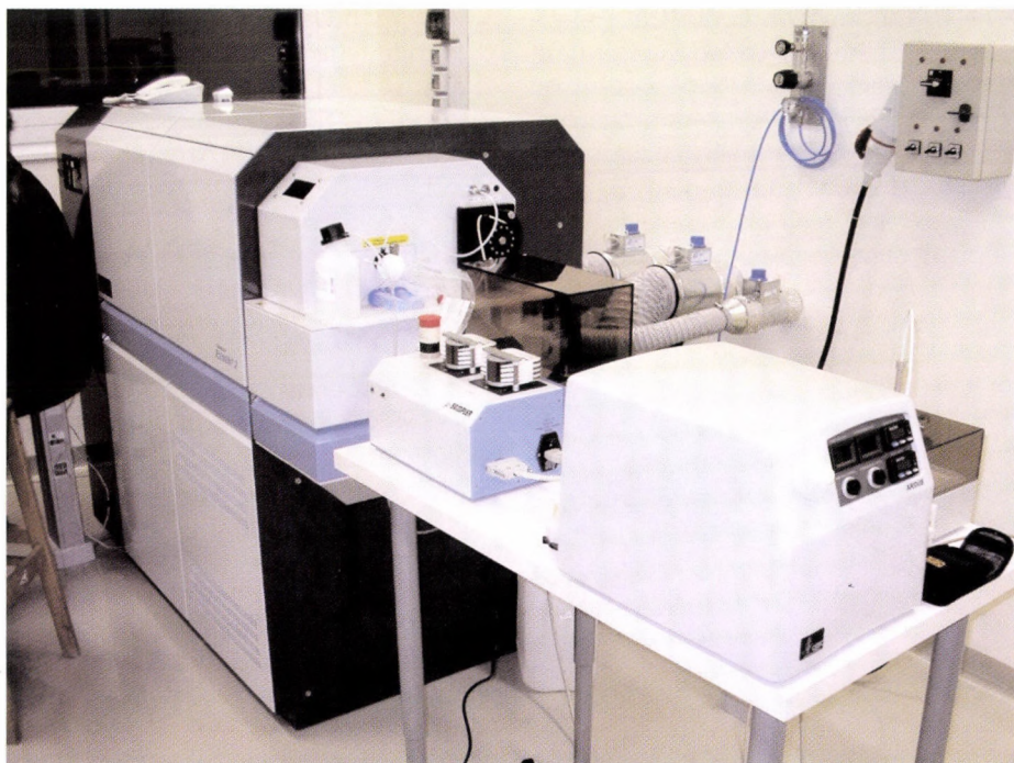
The high resolution ICP-MS with double magnetic focussing equipped with laser ablation option for analysis of isotopes of nuclear materials
