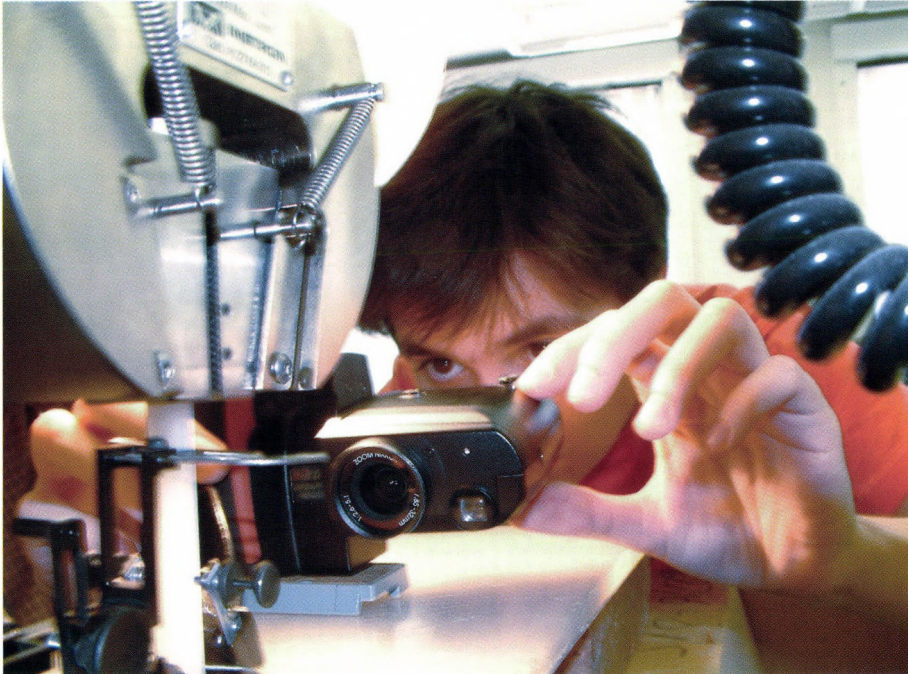
Measuring the acoustic emission of polymers during tensile test
