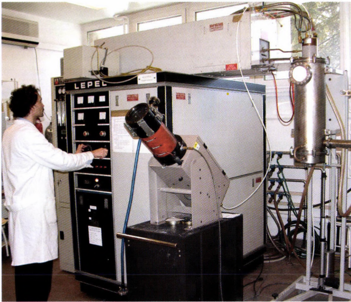
RF thermal plasma reactor for materials synthesis and waste processing
