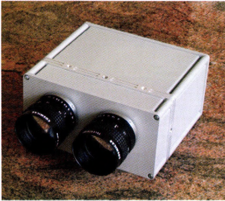
The Bi-i vision system with the CNN chip
