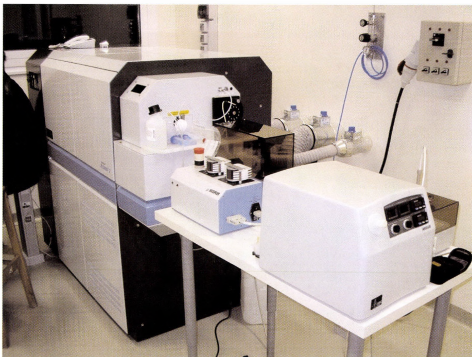
Ion current plasma spectrometer combined with mass spectrometer for analyzing trans-uranium isotopes
