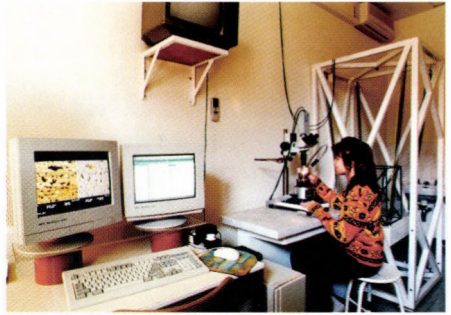
Atomic Force and Scanning Tunneling Microscope for study of surfaces and nano-structures
