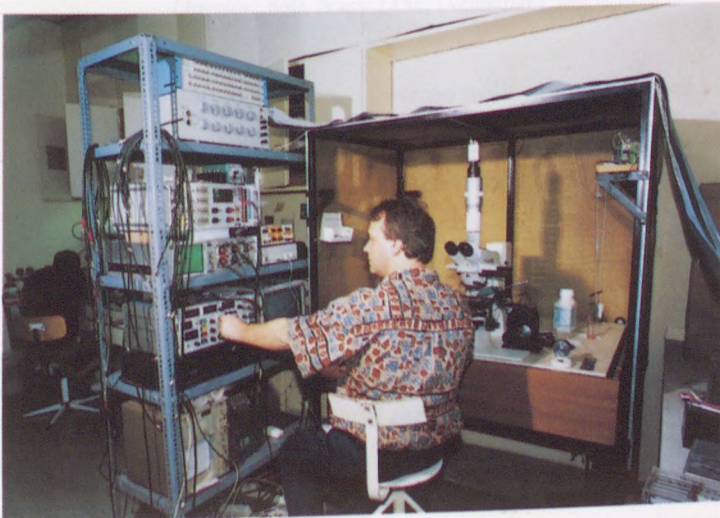
Patch-clamp recording from GABA-containing inhibitory neurons, from in vitro hippocampal slices, visualized by infrared or fluorescence microscopy attached to a CCD camera
