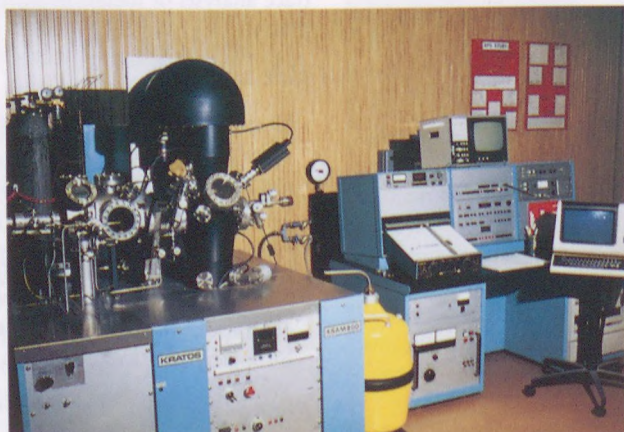
The X-ray Photoelectron Spectroscopy (XPS or ESCA) laboratory dedicated to surface chemical and structure investigations
