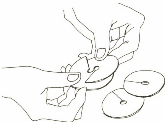
Fig. 3.71. First, the two coloured discs are applied to adjust the \bar{p}_t value: \bar{p}_t = \bar{p}_{t1} + \bar{p}_{t2}
