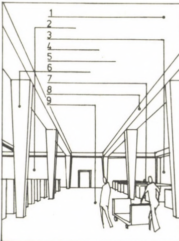
Fig. 5.51. Functionally essential surfaces in an industrial workshop hall: 1) ceiling; 2) wall; 3) wall; 4) door casing; 5) door leaf; 6) pier; 7) machinery, equipment; 8) air ducts and air conditioning equipment; 9) floor
