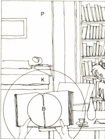
Fig. 5.67. Visual fields of a reading person: B inner visual field, K environmental visual field, P peripheral visual field
