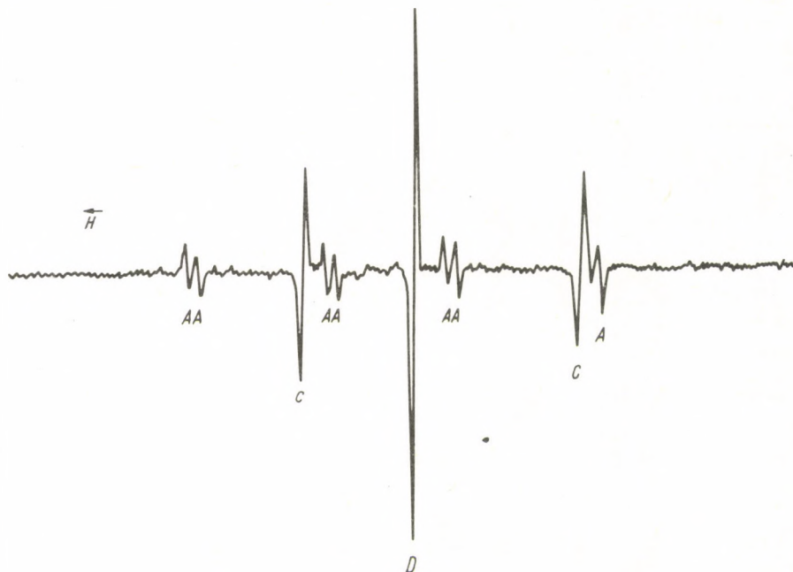
Fig. 8.4. ESR spectrum of radicals originated in photolysis of aqueous solution of vnic acid at pH \sim 1.5 and 31^\circ\text{C} . Emission lines A belong to radical \text{HOOC}-\dot{\text{C}}\text{HOH}-\dot{\text{C}}\text{HOH} , equilibrium absorption lines C to radical \text{HOOC}-\dot{\text{C}}\text{H}-\text{CHO} , line D to radical of oxalic acid whose admixture is present in vnic acid [8.7]
