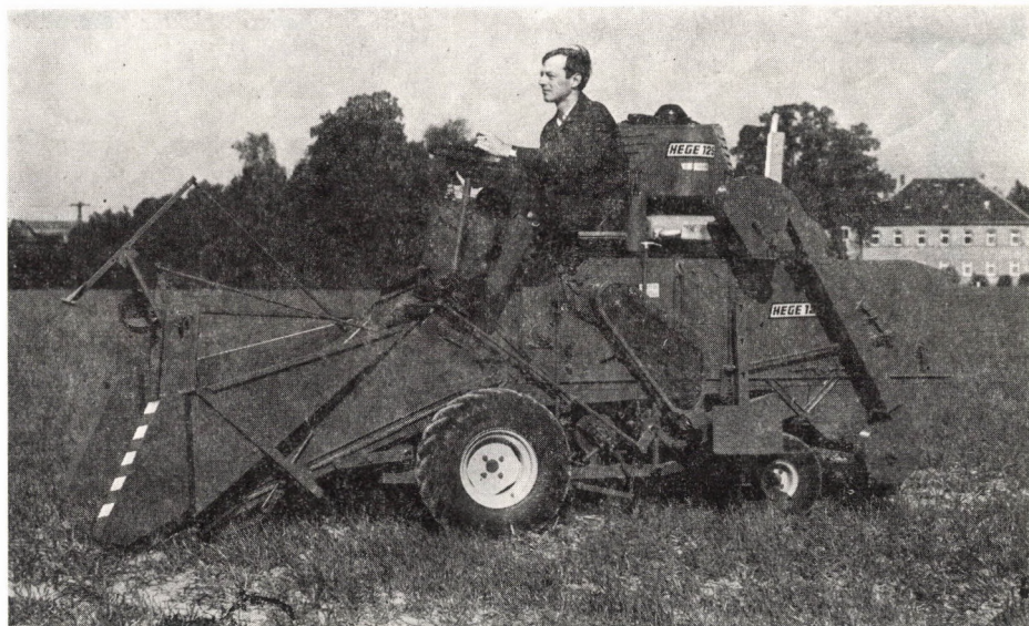
Fig. 54. "Hege 125" type self-propelled plot combine with a cutting width of 125 cm (Hege Saatzuchtmaschinen, Waldenburg/Würt., Austria; photo by Hege)
