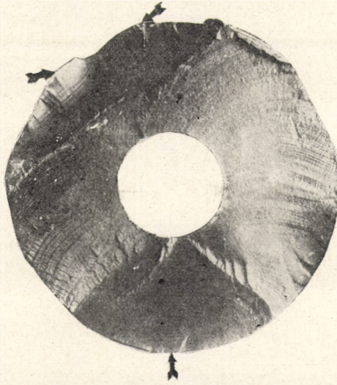
FIG. 1.27. Surface of fracture occurring under reversed bending stress. Failure started on both sides at the positions marked by arrows
