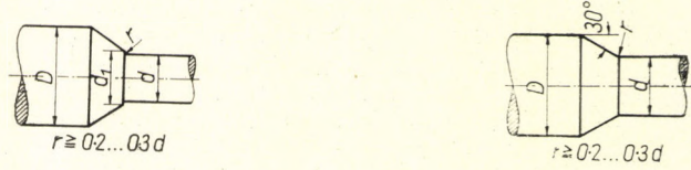
FIG. 8.4. Conical steps in shafts
