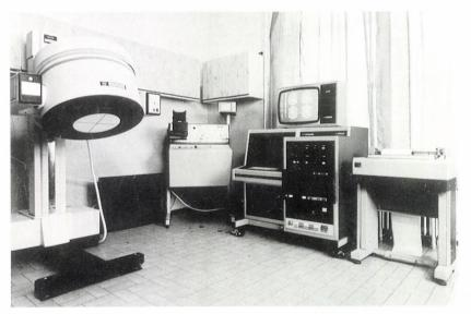
Picture 6.2. Gamma-camera with accessories (GAMMA Művek, Hungary). Left to right: wide-field scintillation detector; electronic signal processor, information processing computer and display unit; graphic printer
