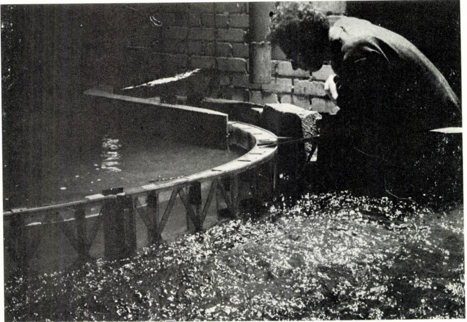
Fig. VI-9. 1 : 20 Hagestein gate model in operation (Courtesy Delft Hydraulic Laboratory, The Netherlands)
