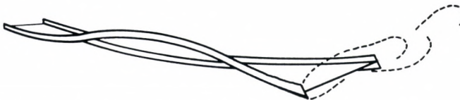
Fig. II-1. Momentary form of road structure of the Tacoma bridge during the gale resulting in its destruction [202]
