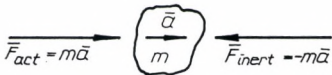
Fig. III-1. Active force \bar{F}_{act} resulting in acceleration \bar{a} of mass m and the d'Alembert reaction \bar{F}_{inert}
